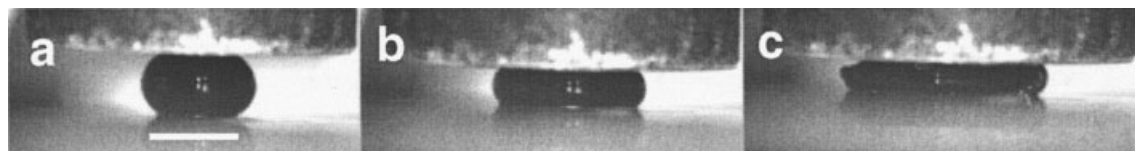
Figure 8 Images of a bead crosslinked with 25 mM genipin and containing sodium alginate in the shell (a) before compression or during compression in the texture analyzer (b) just prior to rupture, and (c) after rupture. Scale bar = 5 mm.
